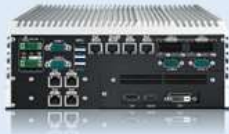
ECS-9200 GTX1050 (Kaby Lake-S + GeForce GTX 1050Ti/1050) 8K resolution, max 7 HD displays & 8 PoE
